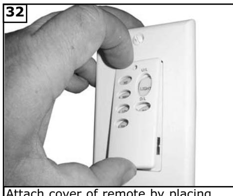
32 Attach cover of remote by placing over buttons and snapping into place.
